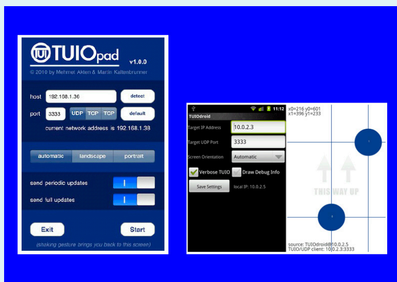
Fig.5 Free apps: TUIOpad used for iOS devices (left), TUIOdroid used for Android devices, such as Samsung Galaxy phones or tablets (right)
